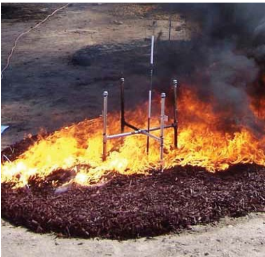
▲ Figure 4. Rubber mulch produced the greatest flame height and temperature of the mulch treatments evaluated in this study.
